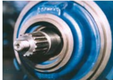
Axle drive shaft for GTWS 1540 / 204
