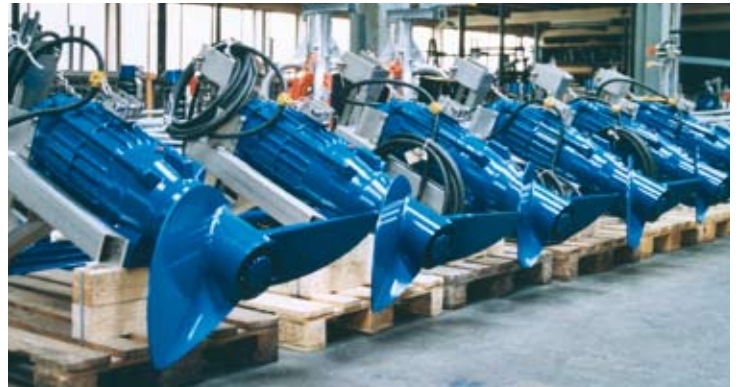
Submersible mixers GTWS 1540 / 204 ready for dispatch
