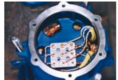
Electrical connection through connector block
