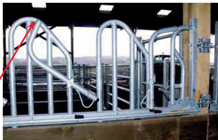
The yoke control bar in the low position and protected by the yoke upright. Very flexible to use.
