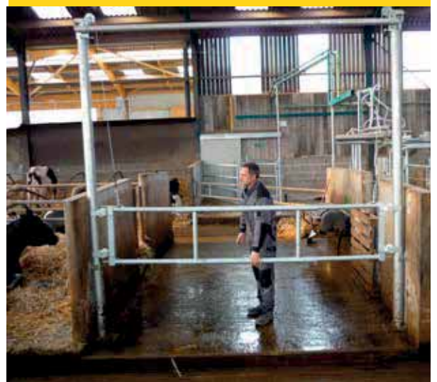
2 rail barrier fitted with 4 nylon wheels with guiding to limit friction
