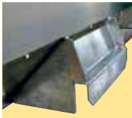
3-point hitch reinforced by a very thick bolted plate
